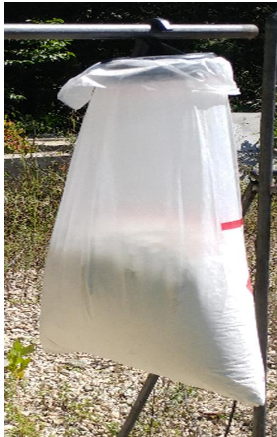
Figure 2.5: Stone Dust Filled Bag and Hook Hanging from Test Stand [35]
