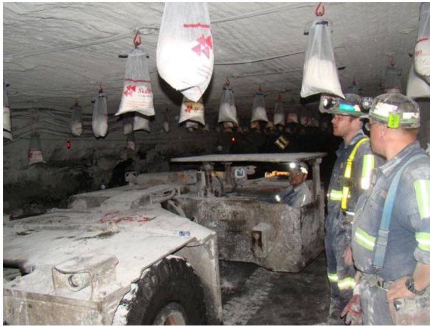
Figure 4.6: Scoop Car versus Bag Barrier Clearance
