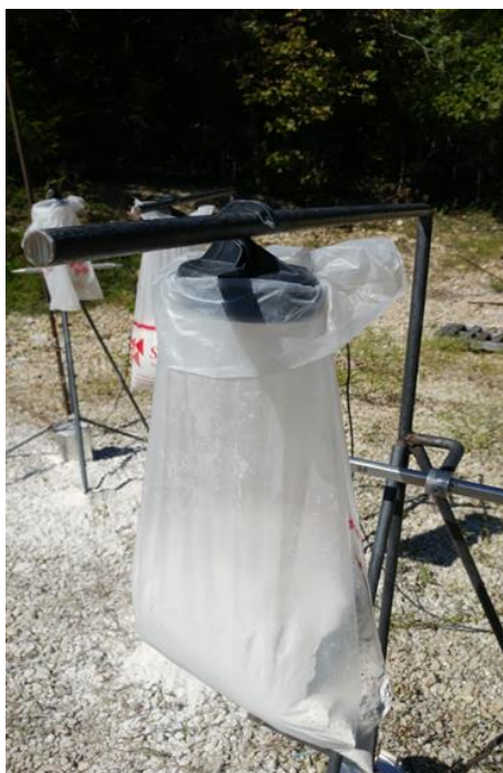
Figure C1.2: 120g C4 Test Bag Position 3 (9 ft)
