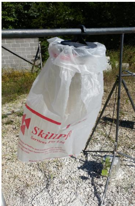
Figure C1.1: 120g C4 Test Bag Position 2 (7 ft)
