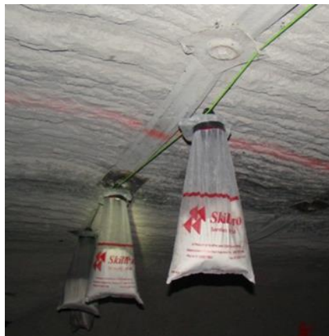
Figure 4.3: Bolt Plate/Cable Support Method
