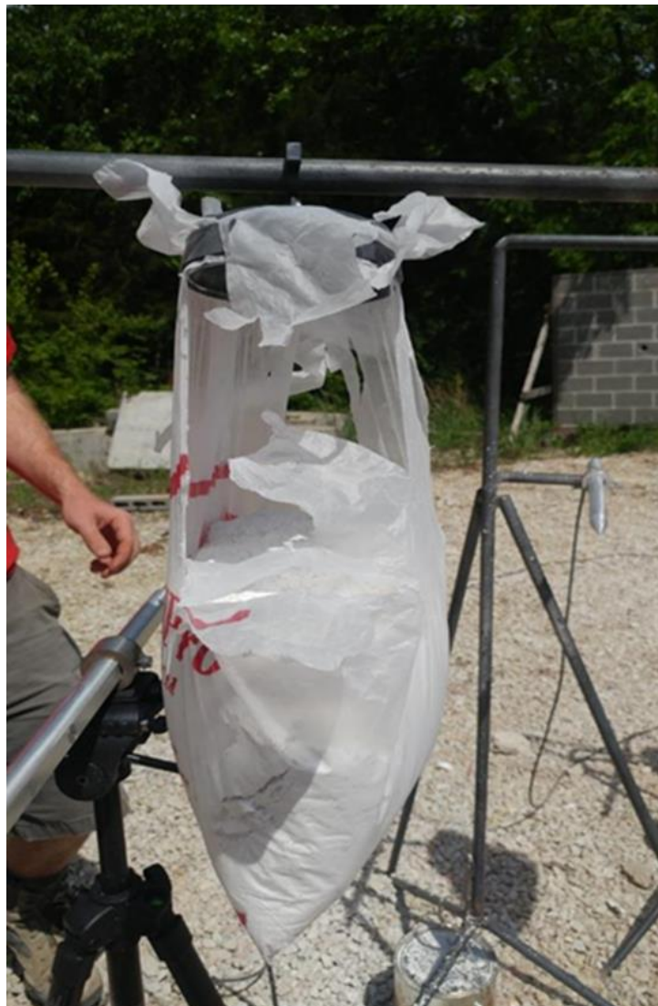
Figure C1: 60g C4 Test Bag Position 1 (5 ft)
